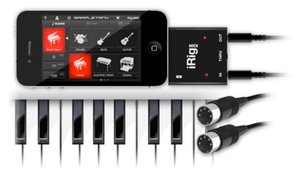
iRig MIDI can connect any standard MIDI equipment such as keyboards, drum machines, drum pads, pedal boards and more to an iOS device to control the included SampleTank FREE\* and a world of Core MIDI compatible apps, such as GarageBand™, available on the iTunes App Store. With iRig MIDI, you can also use iOS apps to control external equipment such as sound modules, digital audio workstations or even lighting systems right from the mobile device.
