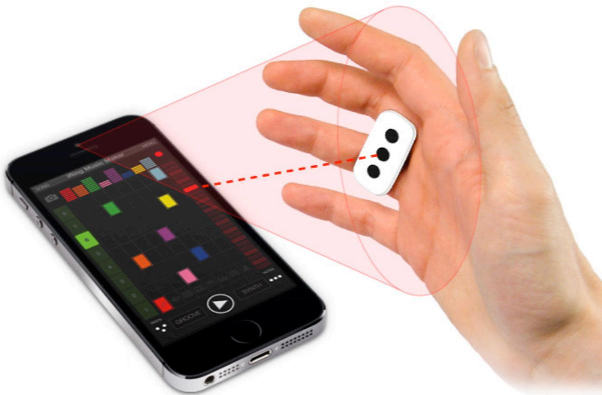
iRing utilizes a wearable ring with identifiable markers, the mobile device's front-facing camera, and advanced computer vision with highly-optimized recognition algorithms built-in to an app, to determine the precise positioning of the ring markers, tracking their movements and position on the 3-dimensional space in front of the device. This system provides a low-cost solution and a motion-tracking device that is accurate and affordable to anyone.
