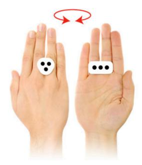
While there have been previous attempts to use a device camera to track hand positioning, they proved not to be reliable for real-word usage, due to the many variables involved in computer vision recognition and the available processing power of mobile devices. iRing solves these issues providing an accurate method for precision detection of hand position in a wide range of lighting conditions.
