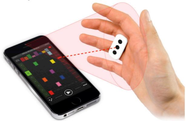
iRing utilizes a wearable ring with identifiable markers, the mobile device's front-facing camera, and advanced computer vision with highly-optimized recognition algorithms built-in to an app, to determine the precise positioning of the ring markers, tracking their movements and position on the 3-dimensional space in front of the device. This system provides a low-cost solution and a motion-tracking device that is accurate and affordable to anyone.
